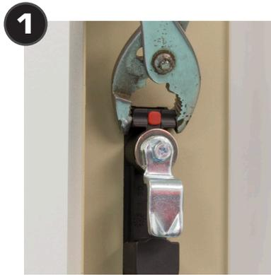
1 From inside the cabinet, use pliers or vice grips to pinch the snap wedges on both sides of the top. While holding both sides in, work the top of the lock assembly loose by rocking side to side and holding the handle on the front of the cabinet.
