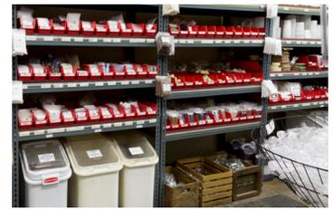
7. Straight Wall Containers are designed to maximize storage capacity on shelving, pallets, and trucks. Because their walls are straight, there is no space lost to tapering or internal "posts" that you might see in a nesting container. This allows for better use of cubic space thus saving customers money on storage and shipping costs. Customers who use Straight Wall Containers vs. Nesting Totes for shipments save approximately 10%-15% over time.
